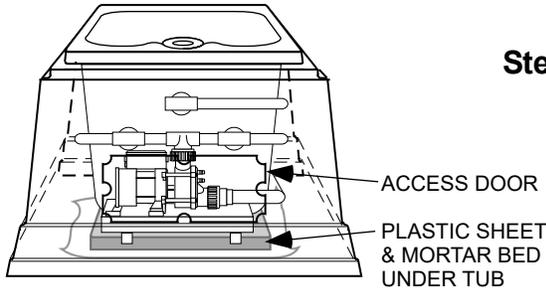
**Step 2.** Look through access door on both ends of the tub to determine how much mortar will be needed to fill the entire area under the tub floor. When the mortar is put into place it will fill the entire area between the tub bottom and the floor & ensures the tub floor will be solid & never flex.
