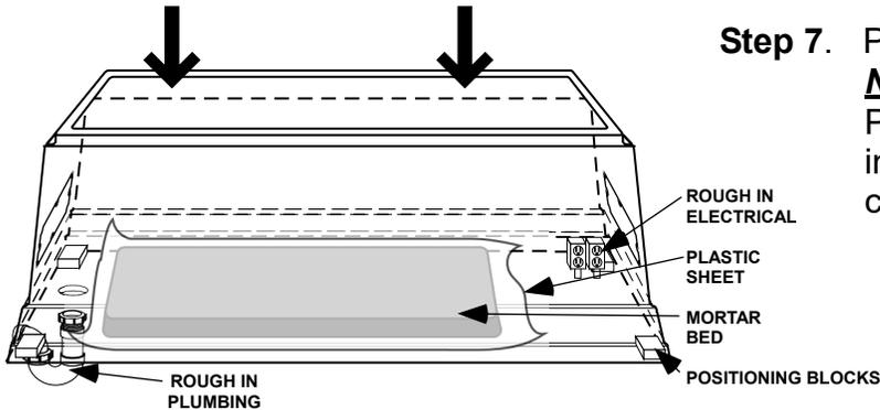
**Step 8.** Hook up all electrical & plumbing after the mortar has fully hardened.
