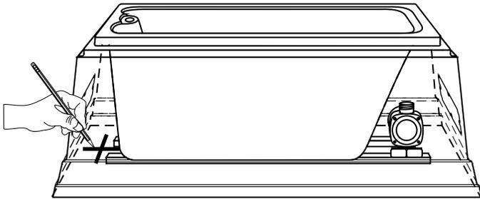
**Step 3.** If rough in plumbing and electrical are already in place, check to be sure everything is positioned correctly. Adjust as necessary. If the rough in plumbing or electrical are not in place mark the location on the subfloor where it will need to be installed. (drain, waterlines, electrical, etc...) Drill or cut the necessary openings.
