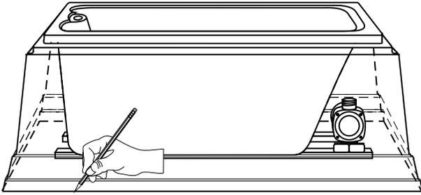
**Step 1.** Place the tub & cabinet in the desired location and outline the perimeter of the cabinet on the floor. Check the tub for level in all directions
