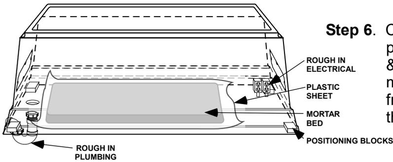
**Step 6.** Cover the mortar with 3 or 4 mil plastic sheet to prevent the mortar from adhering to the tub bottom & allow the tub to be removed if needed after the mortar hardens. Keep the mortar far enough away from the plumbing & electrical to not interfere with their installation or use.
