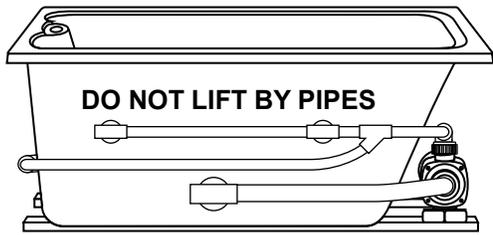
**Step 7.** Place the tub back in the cabinet. ***NEVER*** lift the tub by the pipes or jets!!!! Push the tub into the mortar until it is fully seated into the cabinet and sits firmly and evenly on the cabinet top.
